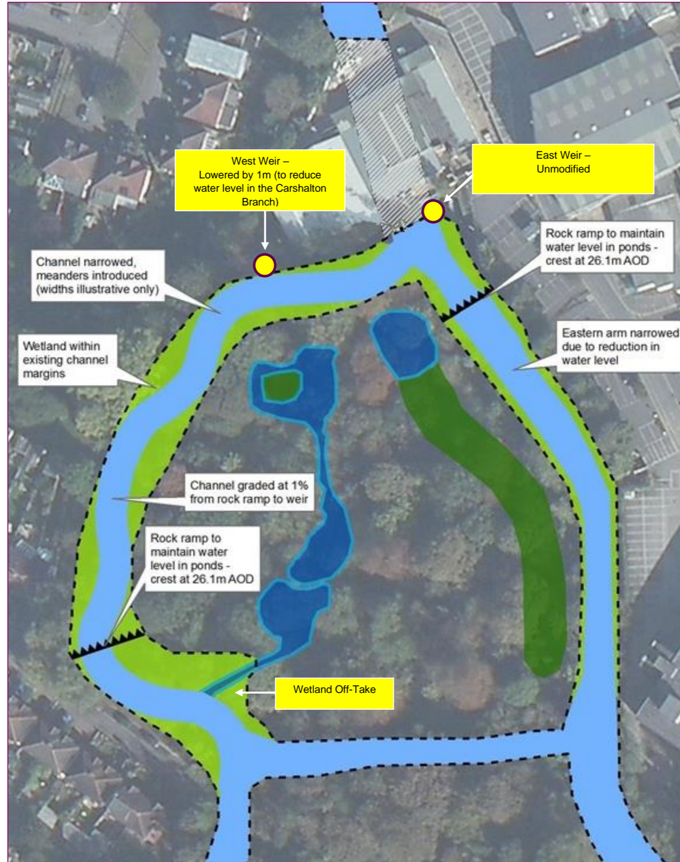
Figure 5.4 Option 4: Weir Lowering and Rock Weirs within the Carshalton & Croydon Branches
