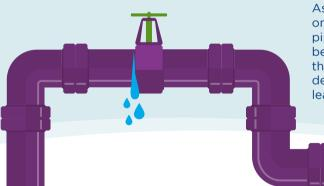
As well as replacing mains that have burst more than once, we use innovative technology to understand which pipes are likely to fail in the future so we can replace them before this happens. The data we collect not only looks at the age of the pipe but also the thickness of its wall - this determines how much it's eroded over time which may leave it more susceptible to future bursts.
